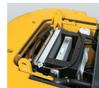
Engine hood locking provides safety servicing
