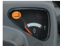
Lifting interlock lamp on the meter panel
