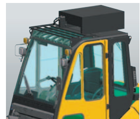
Steel cabin with cooler
