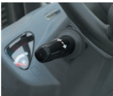
Finger-tip operation with the electric F/R lever
